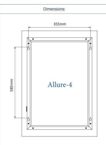
The drawing above shows the dimensions for wall drillings for the installation of the mirror
